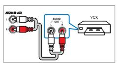
Using an analog cable, connect the AUX connectors on your home theater to the AUDIO OUT connectors on the TV or other device.
